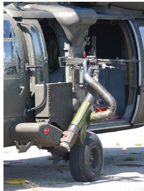
U.S. Army EGMS with High Capacity Feed System, M240
